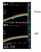
Available in dual transducer configuration for bow and stern transducers. Flexible split screen function can be tailored to vessel specific requirements.
