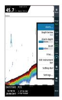
Modern interface is simple to operate and has quick assess to basic tasks such as setting alert depth and changing draft setting.
