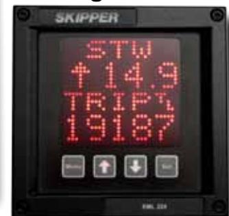
*The SKIPPER COMPACT EML 224 is a single or dual axis speed log, working on the electromagnetic principle, providing longitudinal and transversal ship's speed relative to sea water. The COMPACT EML 224 gives accurate navigation parameters, measured as they happen, and presented in a logical, user friendly way.*
