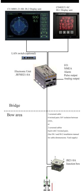
DL21 Doppler Sensor. STW 1-axis sensor SOG 2-axis sensor Installed in 100mm Sea Valve
